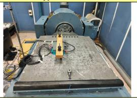
Vibration Test: X axis / Mechanical Shock Test: ±X axis
