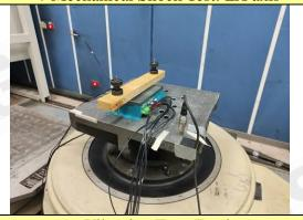
Vibration Test: Z axis / Mechanical Shock Test: ±Z axis
